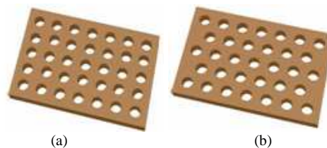
Fig. 1: Examples of photonic crystal slabs. (a) A square lattice of air holes in dielectric (b) a triangular lattice of air holes in dielectric
